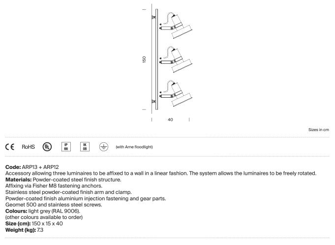
**Installation:** Suitable for wall attachment by means of a fastening accessory. The component is delivered disassembled. The component can be combined with the Arne floodlight product range (for further information about Arne floodlight, log onto the website www.santacole.com).
